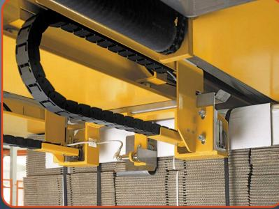
Compression strapping machine for corrugated carton equipped with edge protection applicators to protect the top of edges of the load being strapped.
