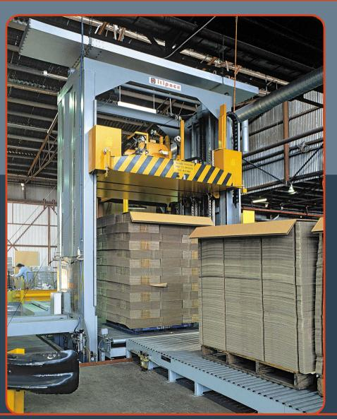
Automatic compression strapping machine for compression till 5 Tons. Equipped with two movable lances to apply the strap through the pallet void; twin heads to apply both strappings and turntable for cross strapping. It has maximum strapping flexibility according to different load dimensions.
