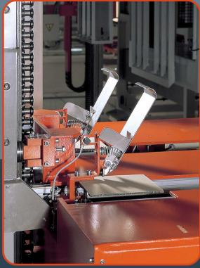
Compression strapping machine for corrugated carton equipped with 4 edge protection applicators, dimensions 200x200x5 mm, to protector the top of edges of the load being strapped. It owns 4 carton edge storages.
