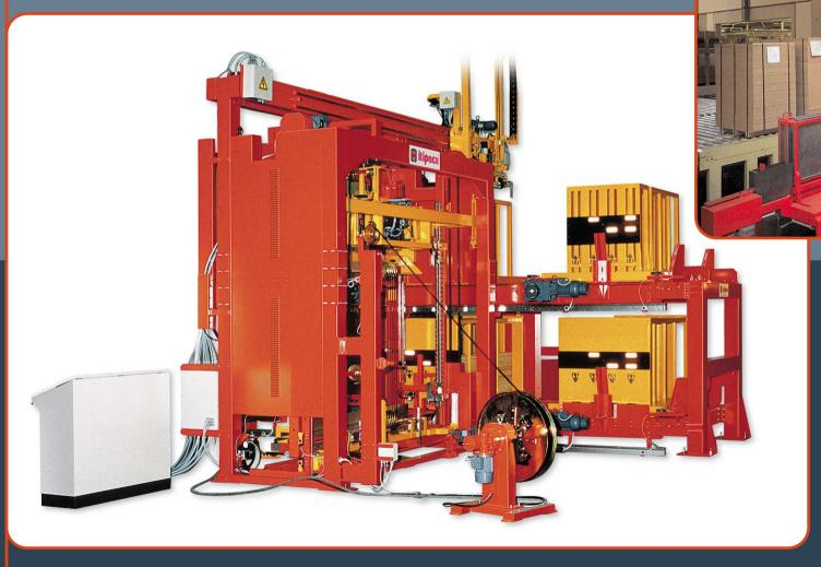
Strapping machine to strap chipboard panels. It is equipped with automatic bunk applicators on 4 sides of package. It is available with sealing head for steel strap or for polyester strap.
