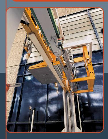
Strapping machine to strap chipboard panels. It is equipped with sealing head for high capacity strap tensioning and device to apply wooden batterns on top of package. It is available with sealing head for steel strap or for polyester strap.
