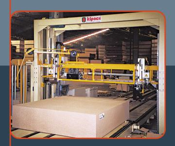
Strapping machine to strap chipboard panels, equipped with high strap tensioning system, with bottom automatic bunk applicators with powered magazines, and top edge protector applicators. It is available with sealing head for steel strap or for polyester strap.
